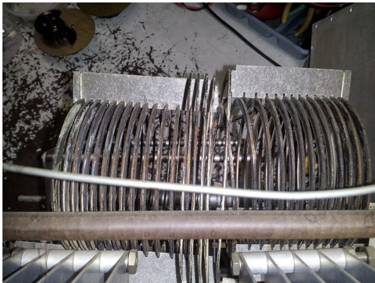
Coil Form Broken In Three Places
